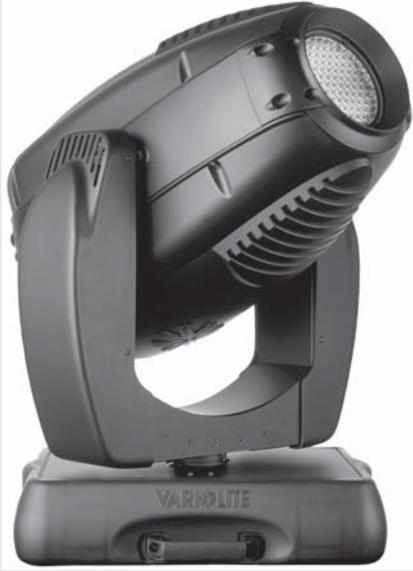
The VARI\*LITE VL3000 Wash luminaire features 6:1 zoomable beam spreader optics, CYM color mixing, variable CTO color temperature correction, a six-position color wheel and separate dimmer and ultra-fast strobe mechanisms. A standard palette of colors is provided with the unit. Custom colors are available.
